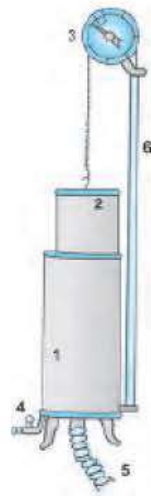
Figure 2-4: Simple spirometer. 1: Outer container; 2: Gas float; 3: Calibrated pulley with spring-mounted indicator needle; 4: Tap for draining water; 5: Wide-bore inlet tube; 6: Counterpoise system
