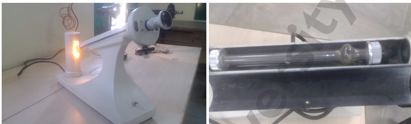
Figure 1: Left-panel : Polarimeter instrument and its set-up. Right-panel : Place of the solution tube in the instrument.
