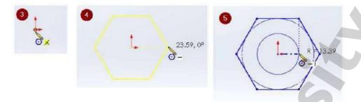
4. Now we will assign dimensions to our outline. Make sure we are still in sketch mode by looking at the top left corner and seeing that the Sketch button is depressed and now reads "Exit Sketch". Press the "S" key on the keyboard. In the small window, click the "Smart Dimension" tool.
