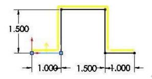
4. Use Line >, sketch and connected open end of this sketch and make it close both end.
