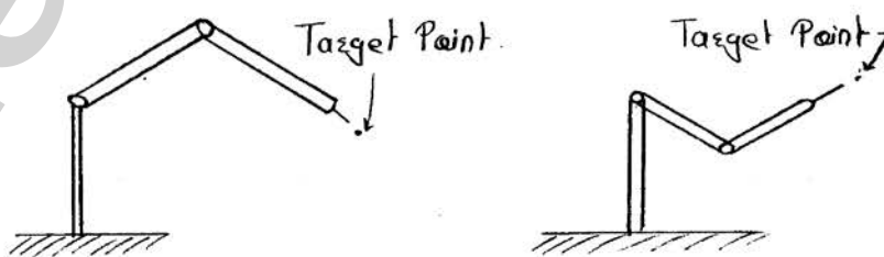
Fig @. → Two alternative axis configurations with end effector located at desired target point.
