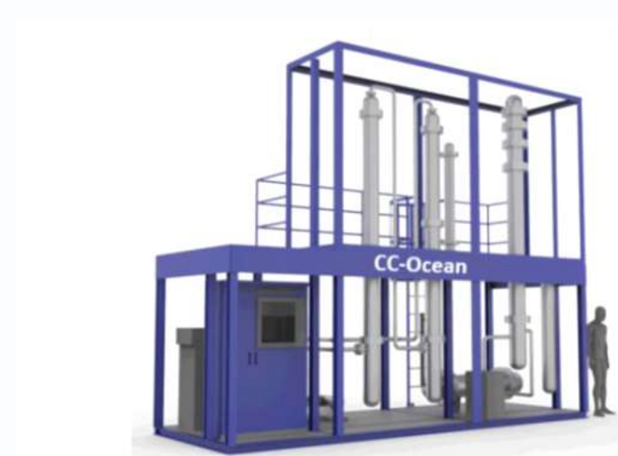
Figure: Small Scale CO 2 capture demonstration plant
