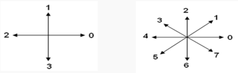
Fig- 4 (a) 4-connectivity (b) 8-connectivity
