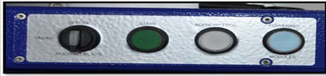
Fig. 1.21- Local mode machine control
