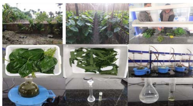
Figure 1: Cost-effective Steam Distillation process for extracting Betel Leaf Oil (BLEO) from 'Sada Bangla' cultivar.
